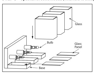
Insert the glass panel into the base. Install the specified bulb type and wattage (not included). Slide the glass down.
